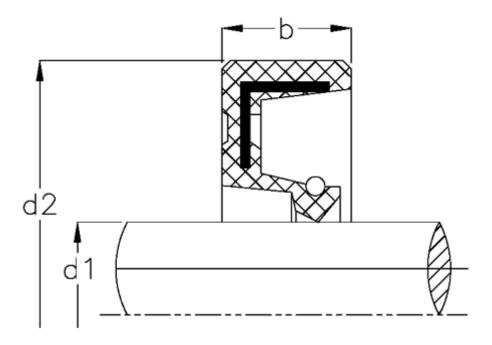
$\begin{array}{ll} b & = 12 \\ d1 & = 62 \\ d2 & = 100 \\ Material = NBR \end{array}$
